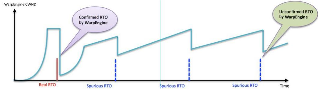
As shown in the image above, if an RTO occurs due to actual congestion, WarpEngine's congestion control behaves as TCP's would to protect against packet loss. However, spurious RTOs caused by jitter rather than actual congestion don't result in throughput collapse, the extended recovery period of reduced throughput, and the loss of available bandwidth that normally follows. As a result, WarpEngine recaptures bandwidth that would otherwise be wasted.
