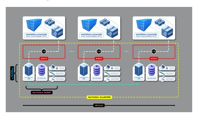
As shown in the image above, one instance of WarpVM is installed with each instance of AHV in the Nutanix hybrid multicloud environment. WarpVM operates under the control of the same management, monitoring, security, backup and disaster recovery features as other applications running in VMs or containers on Nutanix cluster nodes.
